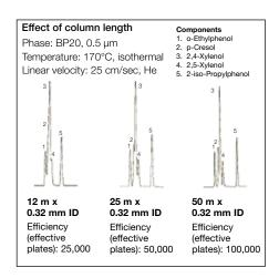
Resolution is proportional to the square root of the column efficiency. Therefore, doubling the column length will only increase the resolving power of the column by approximately 40%.
